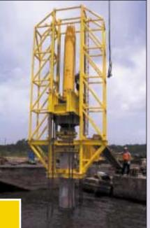
crete piles driven in water depths of 7-12m (21-36ft). The piling contractor, Boh Brothers Construction Company, Inc. of New Orleans, Louisiana assisted AFT in performing Statnamic tests on two piles. The job was performed in two working days. The peak test load on the piles was 4.1 MN. CBK Soils Engineering, Inc. was the Geotechnical Engineer of Record.
